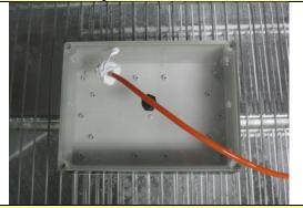
Test for protection against solid foreign objects (Dust test)
