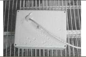
Test for protection against solid foreign 5. objects (Dust test)
