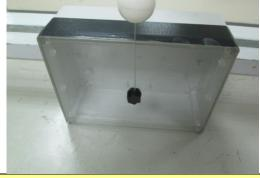
Test for protection against access to hazardous parts
