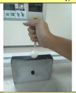
Test for protection against access to hazardous parts
